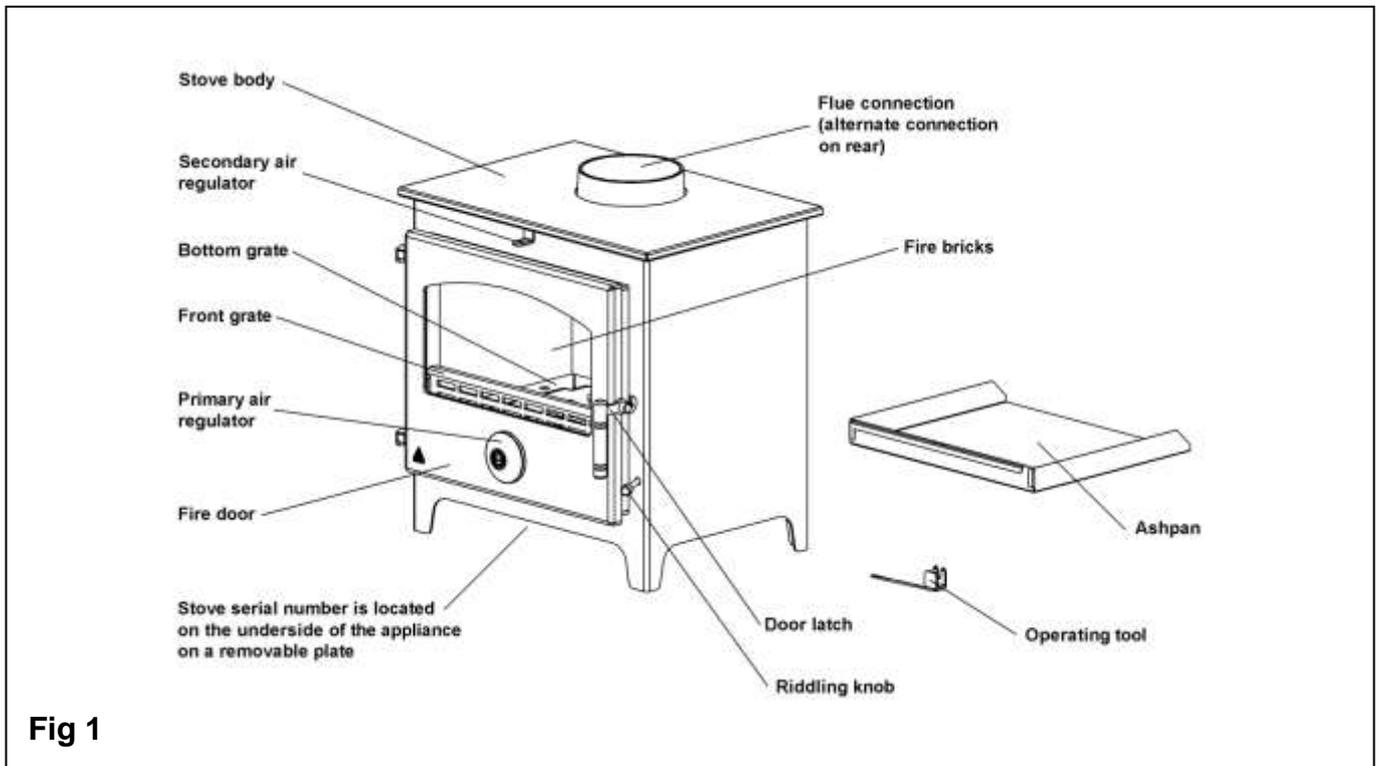
The highest burning rate is achieved by opening the air regulator wheel to maximum. Excess ash formation may indicate over firing.
