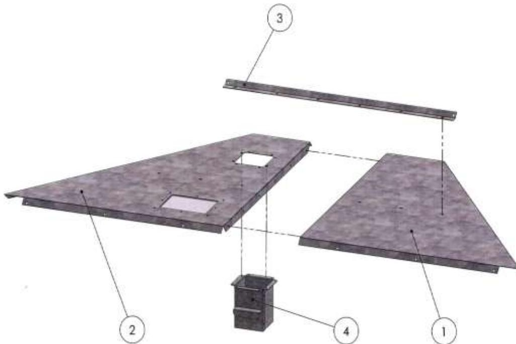
Connect the two chute sections together using M8 x 16 bolts, nuts and washers (6 off).
