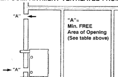
FIG. 6 – VENTILATION FOR ROOM-SEALED BALANCED FLUE BOILERS IN COMPARTMENT BOILER COMPARTMENT VENTILATED FROM OUTSIDE
