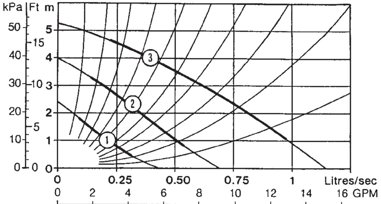
Note: If the pump is run on speed setting 1, domestic hot water availability is impaired.
