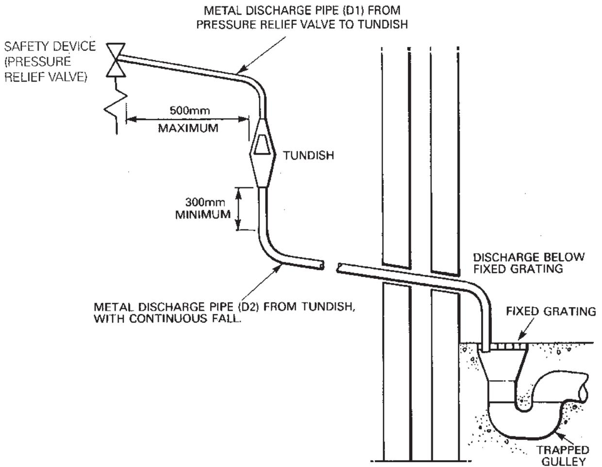
Fig 7 **TYPICAL DISCHARGE PIPE ARRANGEMENT**
