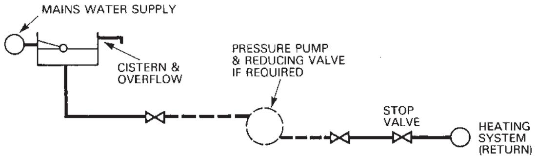
Fig 6 **ALTERNATIVE METHODS OF FILLING A SEALED SYSTEM**
