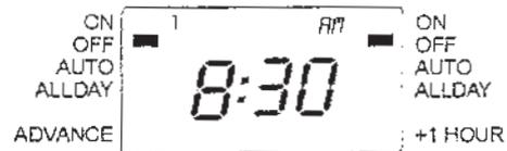
Repeats Steps A, B and C above for event 2 ON/OFF times and again for event 3 ON/OFF times before pressing PROG again to return to RUN mode.
