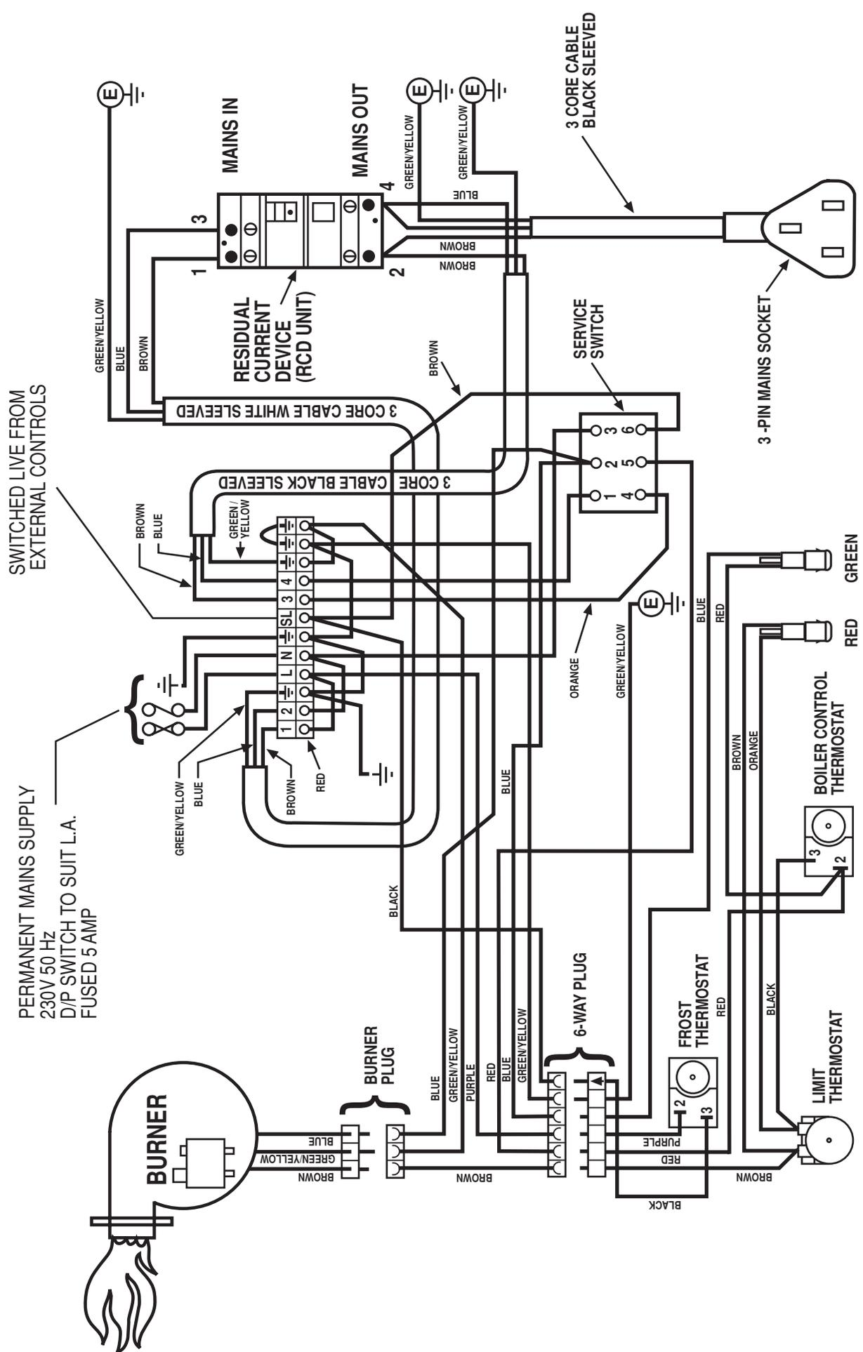
**FIG. 9 BOILER WIRING DIAGRAM**
