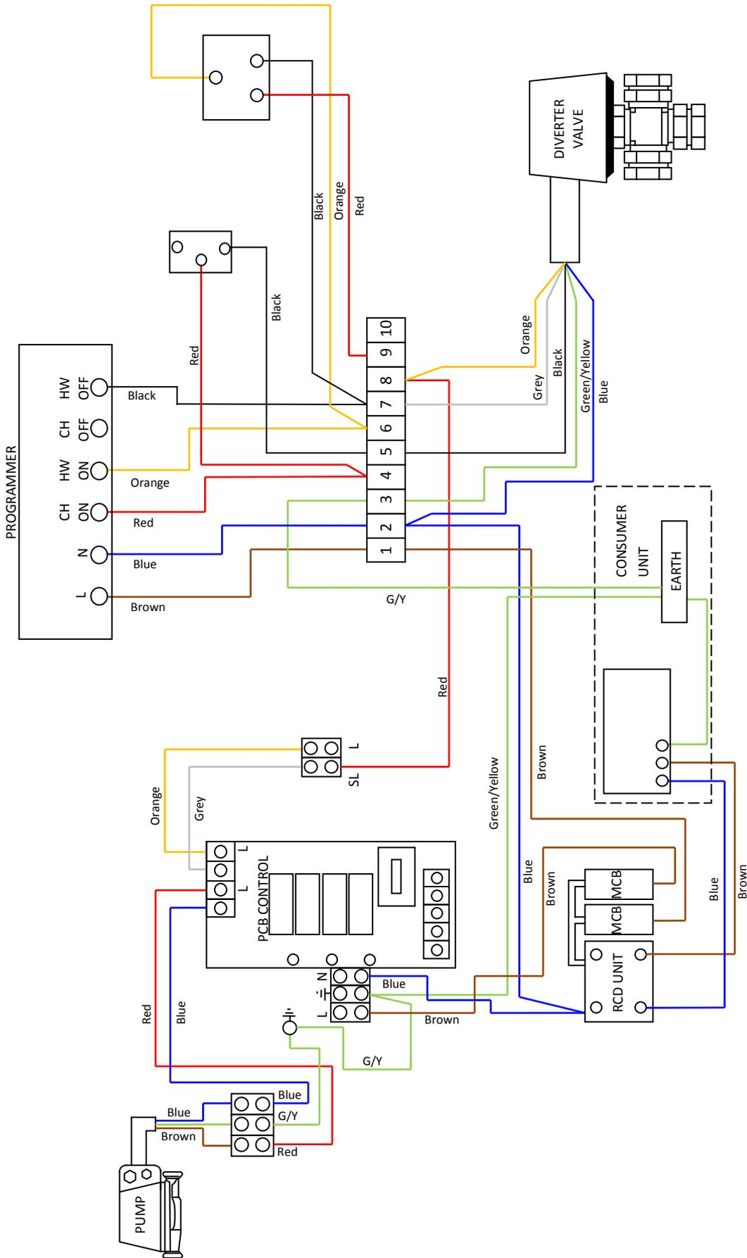
WIRING DIAGRAM FOR Y PLAN CONTROL SYSTEM
