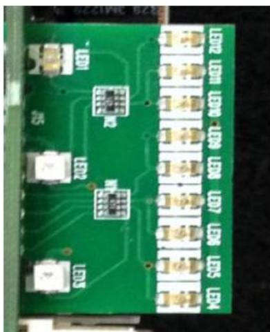
If the red LED light flashes, this means a fault has occurred. This
