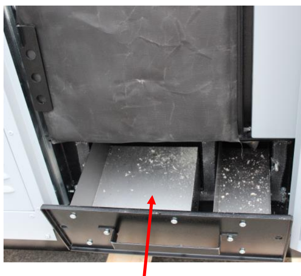
Carefully remove the ash pan and dispose of the ash into a metal container.
