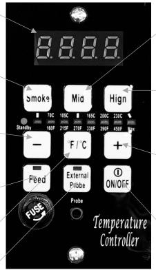
Midrange Temperatures: Sets temperature to 130 °C
