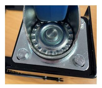
Using the 2 standard wheels locate on to the 2 rear support posts and secure in place using 8 x M8 Bolts, 8 x M8 Nuts and 8 X M8 washers. The bolt heads must be facing downwards when the trolly is in an upright position.
