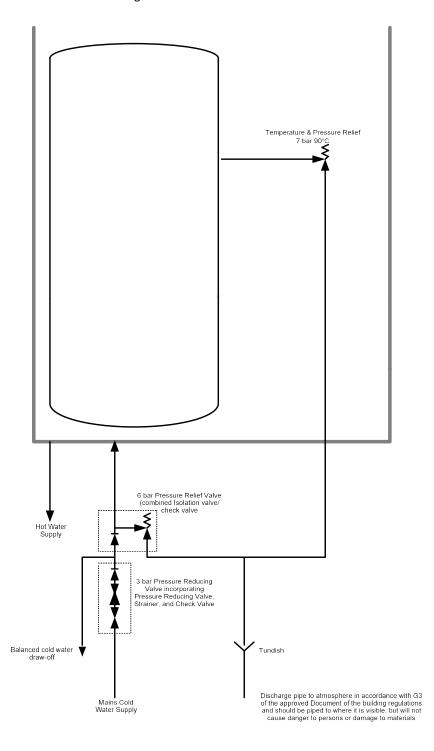
The 6 bar pressure Relief valve, combined isolation valve, check valve and 3bar pressure reducing valve, strainer and check valve are supplied with the boiler and must be installed into the cold mains inlet pipework to the boiler.
