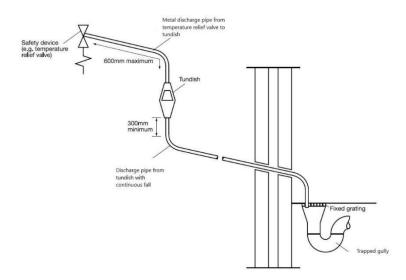
Note: The discharge will consist of scalding water and steam. Roofing felt, asphalt and non-metallic rainwater goods may be damaged by such discharges.
