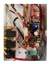
If the boiler displays the F1 code (Overheat) it will be necessary to remove the white panel to expose the circuit boards and disconnect the relay board from the main circuit board by separating the white plug. The boiler will now operate but not produce any heat. Continue with the air removal until satisfied.
