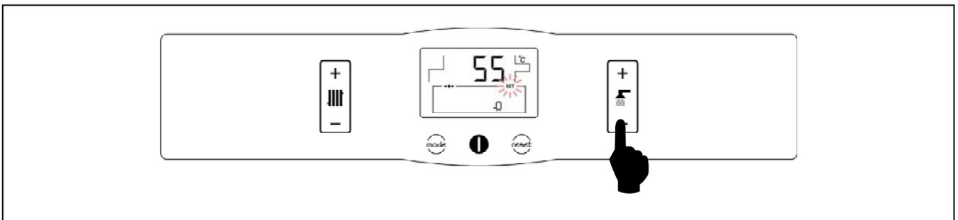
The desired DHW temperature is selected using the touch button, as shown in the figure. To select the desired temperature, touch the "+" or "-" symbols to increase or decrease the temperature respectively. When the temperature has been selected, the display will return to standby mode after a few seconds. The DHW setpoint temperature range permitted is OFF and 30 - 65 °C.
