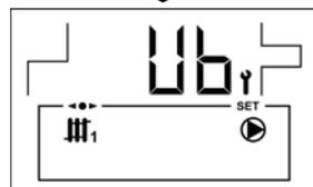
Setpoint of the heating pump speed BC1.
