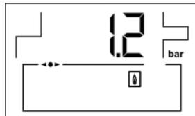
Actual boiler pressure, measured by the Pressure Sensor (11).
