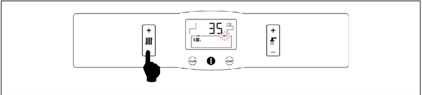
When the boiler is installed with the optional SRFM2/EV underfloor heating kit, the desired flow temperature of the installation can be selected using the touch button as shown in the figure above. To select the desired temperature, touch the "+" or "-" symbols to increase or decrease the temperature respectively. When the temperature has been selected, the display will return to standby mode after a few seconds.
