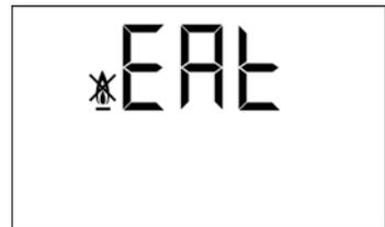
This occurs when the boiler exceeds a temperature of 110 °C. To unblock it, wait until the boiler drops to below 100 °C and press the button on the safety thermostat, located inside the boiler on the underside of the electrical box, after first having removed the button cover.
