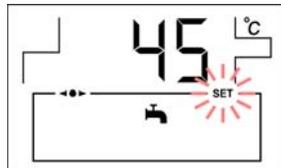
DHW setpoint temperature selected using the corresponding touch button (23).
