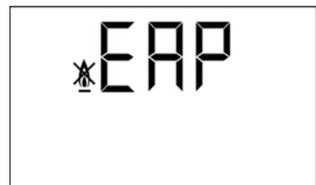
This occurs when the boiler pressure drops to below 0.5 bar, preventing the boiler from functioning when the water is drained from the installation, due to either leakage or maintenance operations. To unlock it, fill the installation again until a pressure of 1 - 1.5 bar appears on the "boiler pressure" setting on the display (18).
