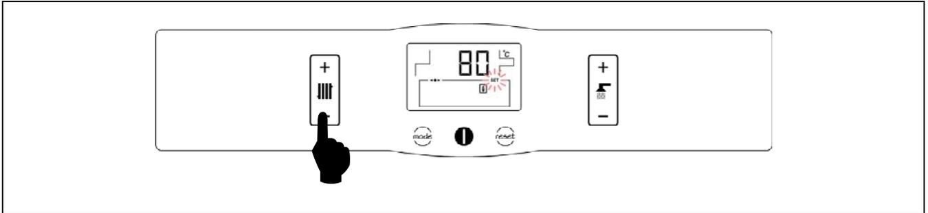
The desired boiler operating temperature is selected using the touch button, as shown in the figure. To select the desired temperature, touch the "+" or "-" symbols to increase or decrease the temperature respectively. When the temperature has been selected, the display will return to standby mode after a few seconds.
