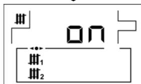
Indication of the heating demand status of each circuit connected to the boiler.
