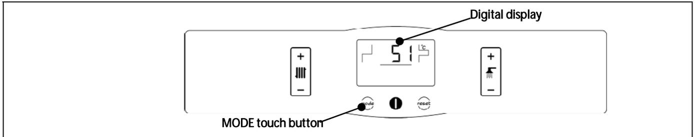
Repeatedly place your finger on the MODE touch button to select the different display options. When the desired option has been selected, it will return to standby after 20 seconds have elapsed.
