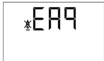
This occurs as a result of an anomaly in the burner (4) or in the fuel installation. To unblock it, press the illuminated button that lights up on the burner.
