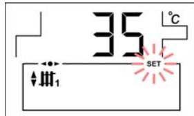
Underfloor heating installation flow setpoint temperature selected using the corresponding touch button (19). (option SRFM2/EV only)
