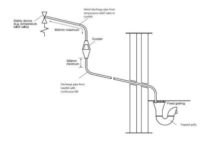
Note: The discharge will consist of scalding water and steam. Roofing felt, asphalt and non-metallic rainwater goods may be damaged by such discharges.
