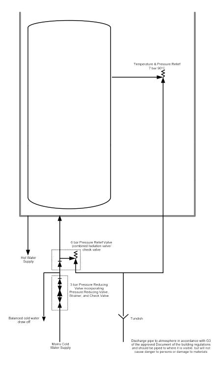
The 6 bar pressure Relief valve, combined isolation valve, check valve and 3bar pressure reducing valve, strainer and check valve are supplied with the boiler and must be installed into the cold mains inlet pipework to the boiler.
